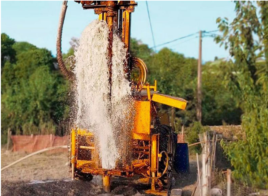
Figure 4. Rotary drilling machine. Source: Hard Rock Drilling - Perforaciones para Obras Civiles [online]. Available at: https://www.hrd.cl/index.php/category/pozos-de-agua/ [Accessed on: 2026]
