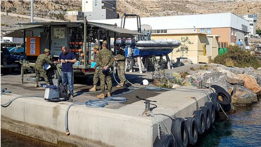
Figure 5. SETA water treatment plant. Source: Refresher course on water purification for sappers from BRI II - Army (defensa.gob.es)
