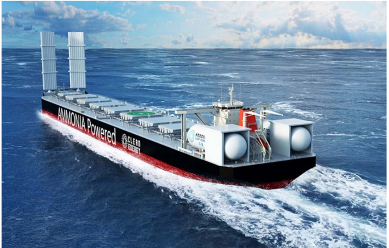
Photo No. 4. Prototype of a vessel powered by ammonia, featuring deck-mounted tanks and solar sails.
