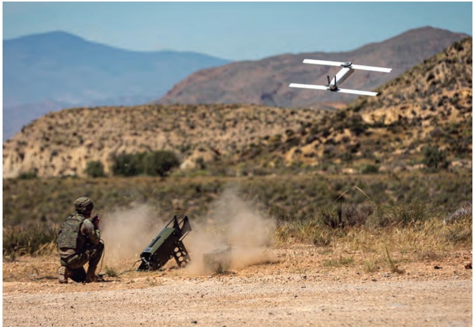
Launch of a Q-SLAM 40 tactical loitering system (kamikaze drone) developed by Arquimea at the Legion's Álvarez de Sotomayor training area in Viator, Almería.
