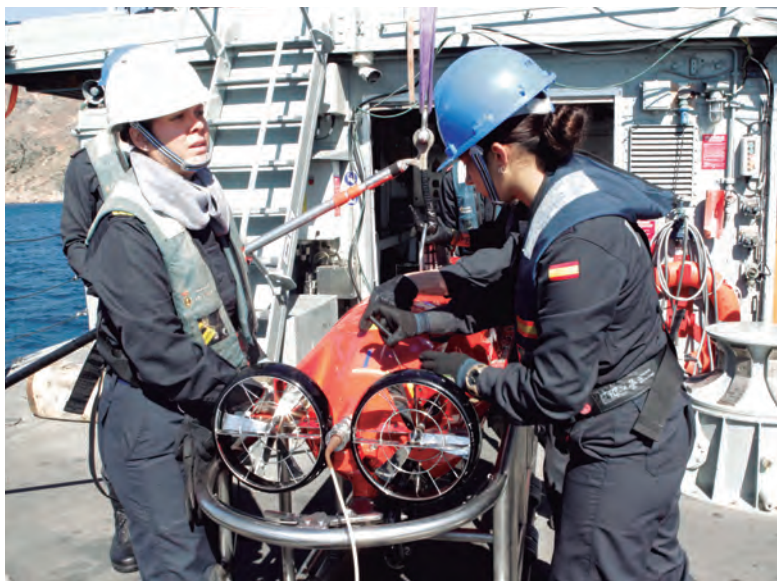
On the deck of the Turia , the crew carries out pre-launch checks on the Pluto Plus before launching it into the water
