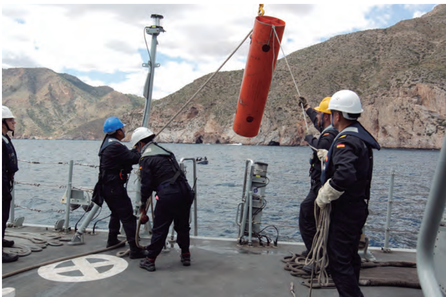
Once located, the Turia 's crew recover the cylindrical mine they were seeking and hoist it aboard using the lines previously rigged by the divers.
