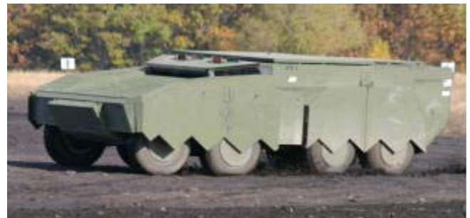
Figura 4. AHED- Advanced Hybrid Electric Drive . CF: Defense Update Magazine
